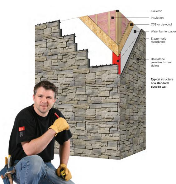
There are no specific structural requirements. You can install the panels inside or outside directly on a partition wall or concrete foundation. If you wish, you can begin by installing compressed panels for better insulation.
